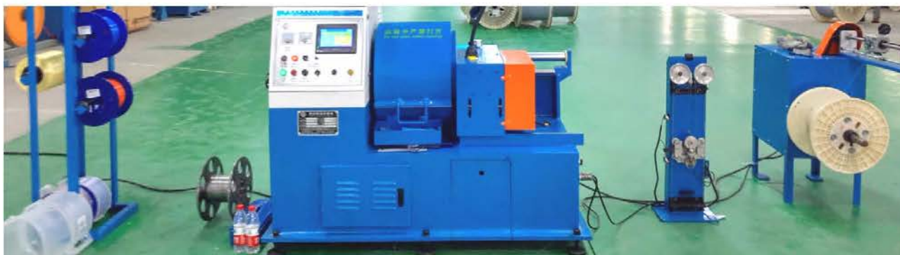
(7) 野战光缆设备(Equipment for optical cable for field operations)
