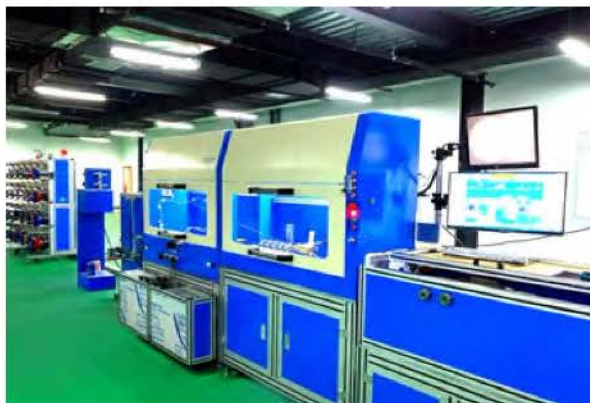
不锈钢管生产焊接设备 Welding equipment for stainless steel pipe
